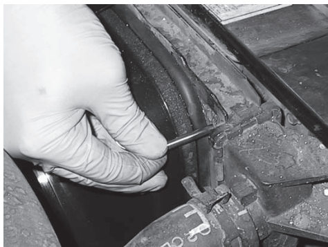
Install temp. probe near inlet hose...
