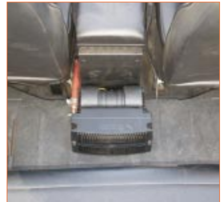
8. The Mojave Heater can also be installed behind the front seats as an auxiliary heater for your rear passengers. We'd recommend that if you use a Mojave Heater as an auxiliary unit, you plumb it in with copper tubing under the body and use small pieces of hose at the ends only. This will reduce your need to reroute heater hose from the motor to the heater every few years.
