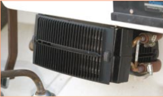
6. The Mojave Heater fits cleanly under the dash, even with the limited space on a flat fender. Some modification of the shifter cane may be required on manual transmission applications.
