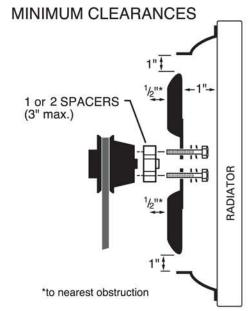
Fan should project into shroud approximately one half of the fan's depth; blade tips should clear lip of shroud by about 1". The fan should not be any closer than 1" to the nearest forward obstruction.
