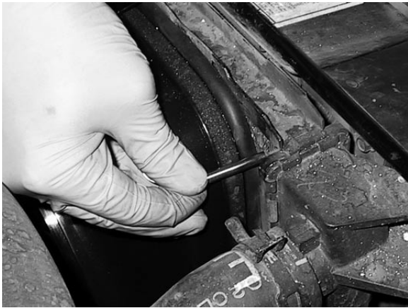
Install temp. probe near inlet hose...
